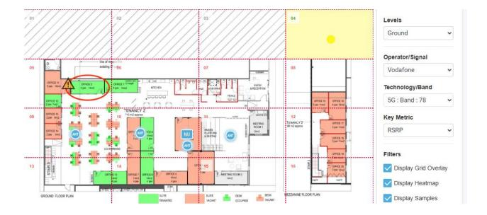
Vodafone Band 78 medium external coverage for donor antenna and would be suitable for upgrading to a G51 repeater to provide excellent internal complete coverage of 5G
